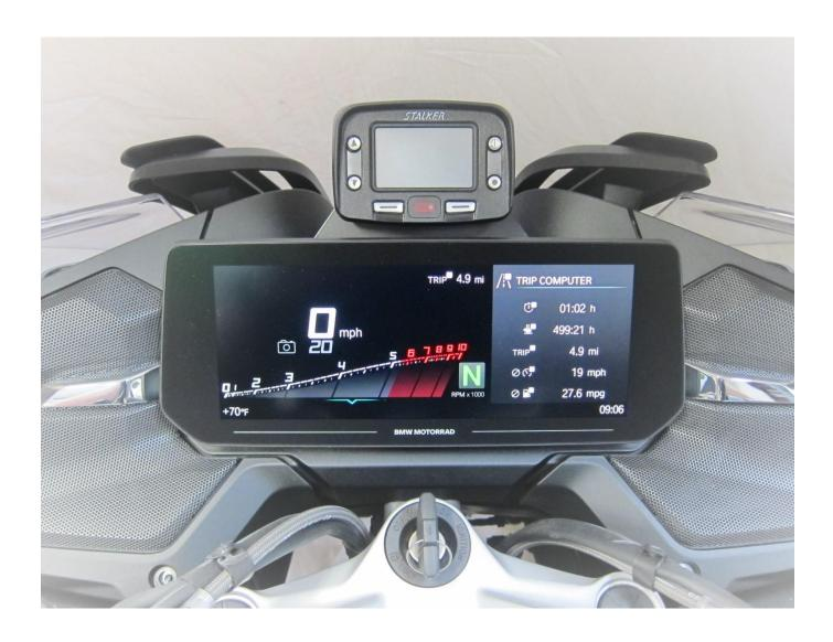
The most time consuming part of installing moving radar is the installation of the display head, as it requires routing the display head cable up behind the instrument cluster. Therefore, remove (or do not install if new unit) windshield and dashboard.
