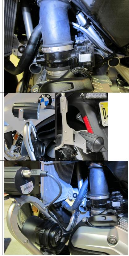
Route the rear antenna cable along the saddlebag frame, up around the forward mount and then up into radio box. Secure the rear antenna cable with a cable tie onto the forward saddlebag frame mount.
